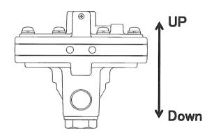
(5)The relay response will be slow when the bypass valve is opened and will be fast when it is closed.
